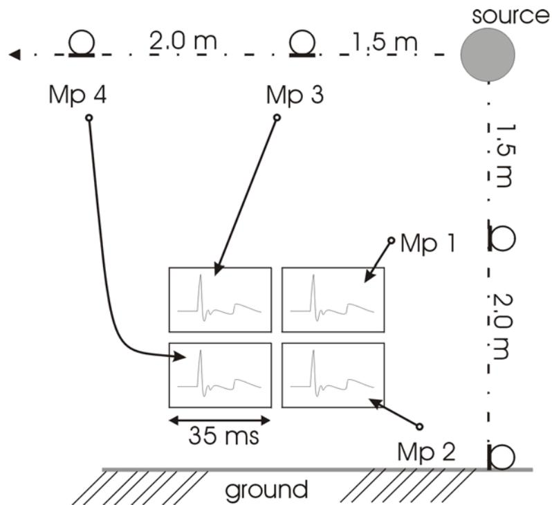
Fig. 1 Basic test plan to measure the absorption and the presentation of pressure time histories used through out this paper
