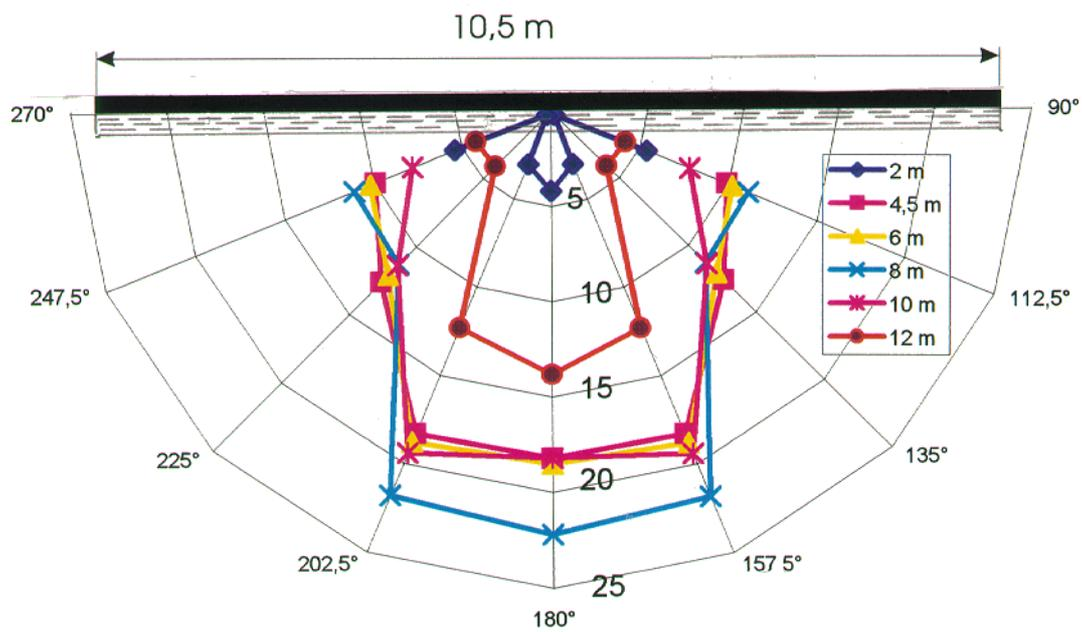
Fig. 20 Level reduction of ASEL for different measuring heights versus reflection angle. Source at 13 m centered in front of the baffle, levels measured on a 20 m radius circle around the center of the baffle
