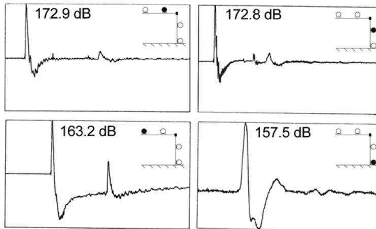
Fig 12 Pressure time histories for the compressed straw absorber, according to fig.11 (scaling see fig. 1)
