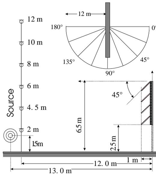
Fig. 14 Measuring layout for baffle reflection into the 180° direction at
