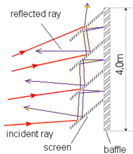
Fig. 15 Sketch of the ray tracing through a 'multiple-screen' design
