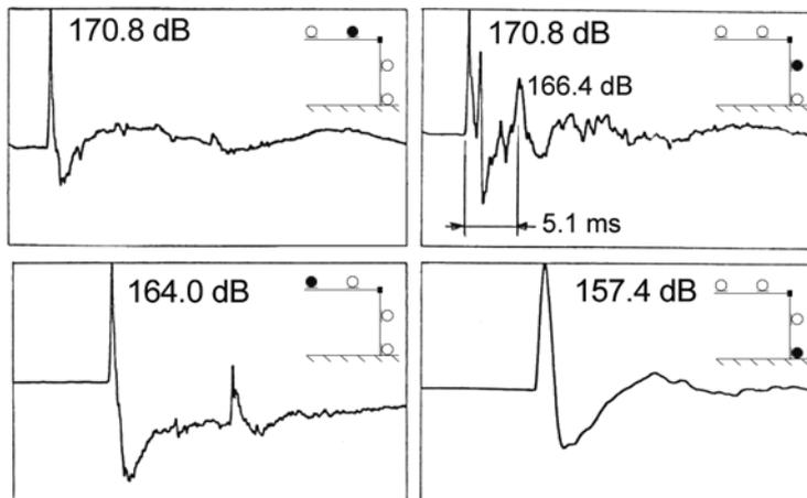
Fig. 6 Pressure time histories for the layered absorber according to fig. 8 (scaling see fig. 1)
