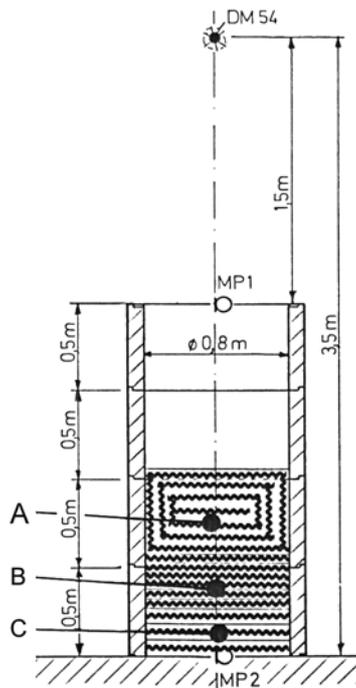
Fig. 8 Tube filled with 3 layers
