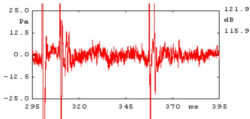
Fig. 17 Pressure time history of the signal measured at 8 m height with a baffle covered with the wooden layer
