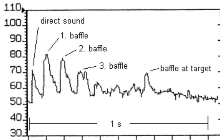
Figure 13 A-weighted level [dB] versus time received at the rear of a rifle range with baffles, distance 300 m
