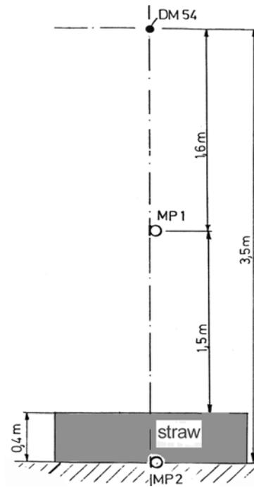
Fig. 11 Set-up for measuring the straw absorber
