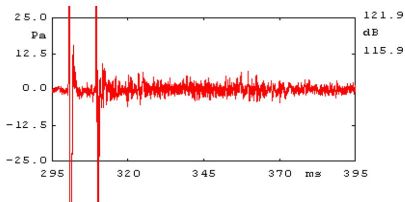
Fig. 18 Pressure time history of the signal measured at 8 m height with a Multiple-Screen-Absorber
