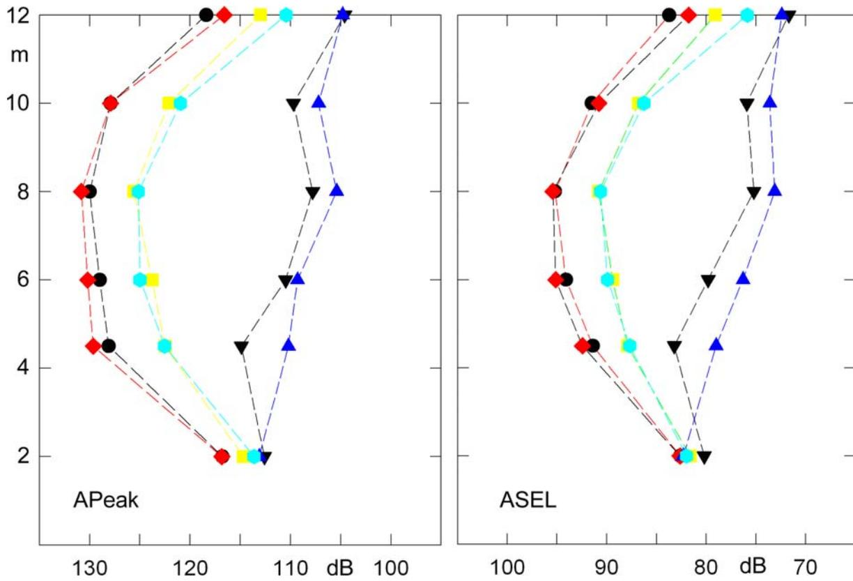
Fig. 19 A-weighted peak level (left graph) and A-weighted sound exposure level (right graph) at 6 receiver heights for the steps of developing a MSA, firing position is 13 m in front of the baffle, 1.5 m above the concrete floor of the test site
