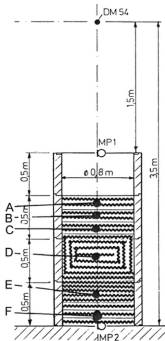
Fig. 9 Tube filled with 6 layers
