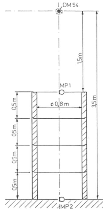
Fig 5 The empty tube including dimensions and measuring positions of MP1 and MP2
