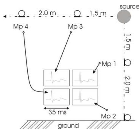
Fig. 1 Basic test plan to measure the absorption and the presentation of pressure time histories used through out this paper
