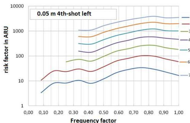
**Figure 7:** Relationship between frequency reduction factor (due to an increased explosion mass) and ARU risk factor
