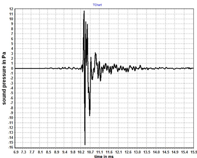
**Figure 1:** Time history of the Z-weighted sound pressure of a pistol firing a percussion cap measured at 0,5m distance by deBAKOM 2012 using EN71-1 [1],  $L_{CPeak} = 119$  dB
