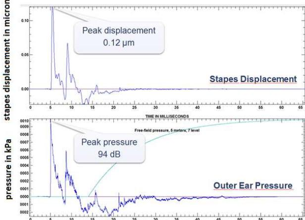
**Figure 3:** Time histories of the stapes displacement (upper part) and of the related outer ear sound pressure (lower part)
